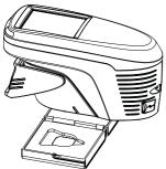
Open the standard box and position the instrument on the white standard. The instrument snaps into the indentation of the standard and can only be positioned in one direction.
